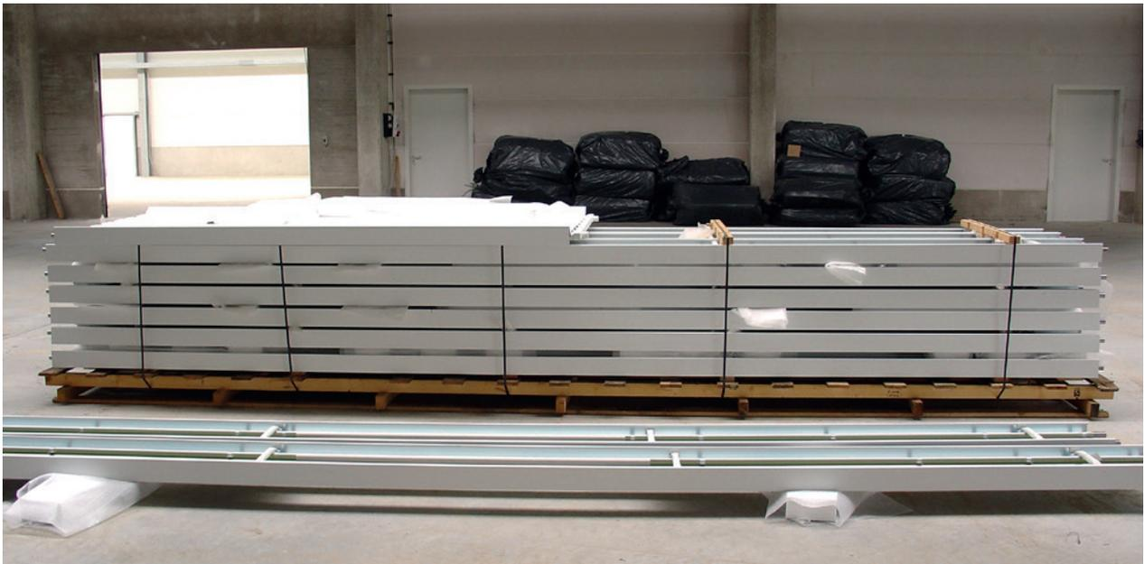
Figure 1. Panels on pallet and bagged insulation
