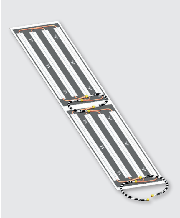
Figure 2. Example of multiple panel runs
