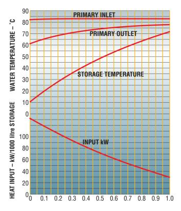
It would also be inaccurate to estimate the heat up time by recording part of the cycle and projecting the time scale in a linear manner. However, the logarithmic curve for secondary rise printed with this leaflet can be a useful guide to the heat up time, using the appropriate portion of the graph for the temperature rise recorded. Remember no draw-off or secondary recirculation can be allowed whilst these measurements are being taken.
