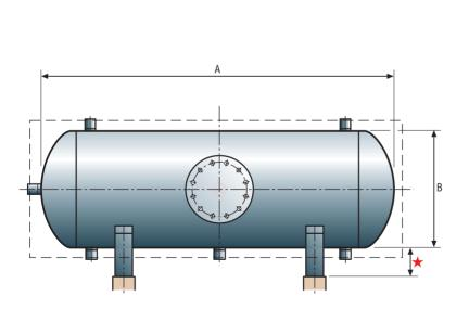
Typical horizontal buffer vessel arrangement.
