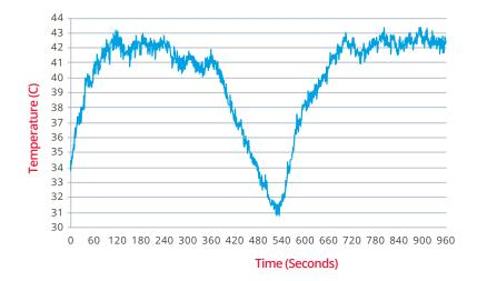
The chart shows temperatures measured on the outlet grille of an SPC fan convector utilising 'Active LST' control. The outlet grille and top panel are the hottest points on the casing.
